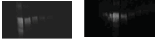
Figure 3: LumiGLO (left) and ECL Plus (right) labelled Western blot image captured by the G:BOX iChemi XR after a 15 minute exposure showing from left to right 500ng, 50ng, 5ng, 500pg and 50pg of human IgG.
